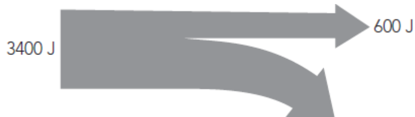
Figure 4.52: Sankey diagram for a coal-fired locomotive.
