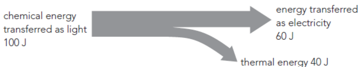
Figure 4.50: Sankey diagram for a solar cell.
