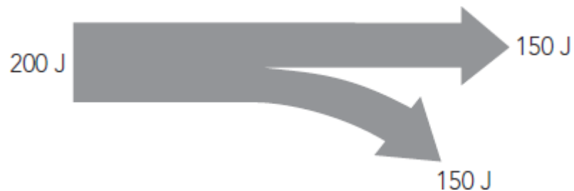
Figure 4.53: Sankey diagram for a lamp.
