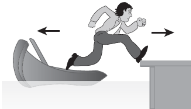
Figure 5.12: As the person jumps out of the boat, the boat moves away from the shore.
